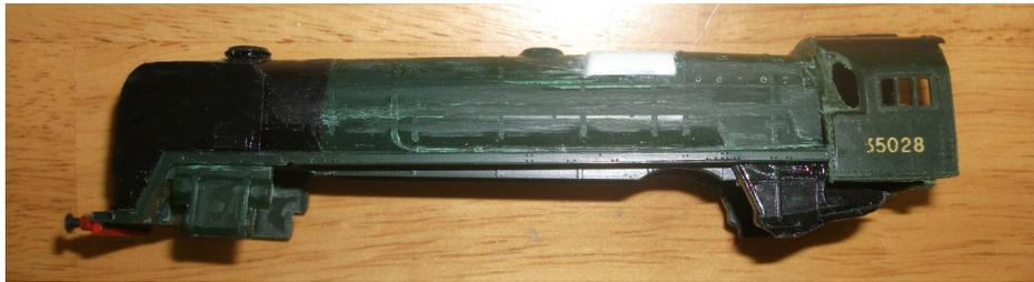
As can be seen, when the main cab portion is positioned the roofline is well out of height. This issue was rectified by removing the roofline as shown in the image above, and inserting a new roof, made from plasticard into the gap created by the roof's removal.
