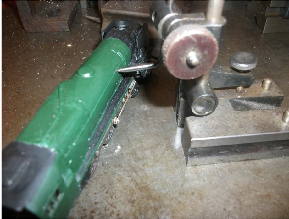
The scribed line gives the required height. Once this was marked, I used a pair of dividers to scribe the position of the stanchions. Using the dividers as opposed to a rule had one major advantage in the fact that the measurements would be identical on either side of the body.
