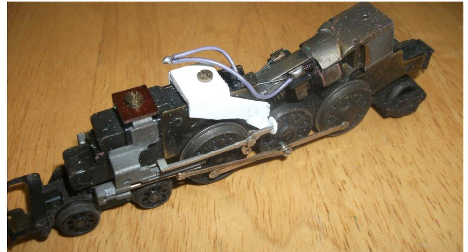
To avoid some of the issues associated with the Britannia bracket, this was made up using 2 layers of Plasticard sandwiched together to create stronger joints, with fillets being used to strengthen up the other components.
