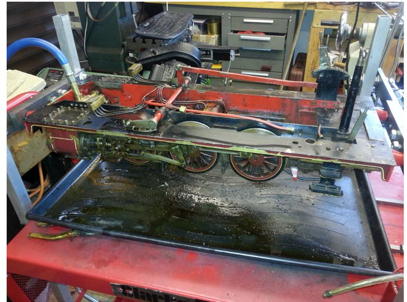
My adaptors require the buffers to be removed, as I suspend the engine using inserts in the buffer housing at each end of the locomotive. I have adjustment screws on beams at each to ensure the engine is securely
