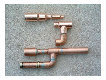
The venturi is assembled from readily available plumbing fittings, and the photograph above shows both a complete assembly, and most of the component parts laid out alongside. The parts are as follows:
