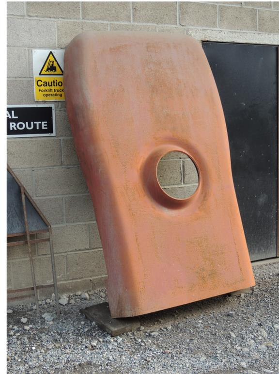
We were also shown their press that they use for shaping boiler plates, and we were told that when they set up to press a plate, they always press at least 2. A second, in case they make a mistake with the first one, but often a third which can be sold later. We saw several examples of back-heads in the yard outside, one of which is shown here.
