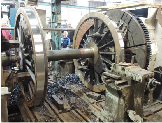
The majority of their contract work is on wheel-sets, and we saw this pair, mounted between centres, for turning the wheel tread.
